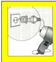
This plug has two round pins and is for use in parts of Europe, Middle East, and Asia.
