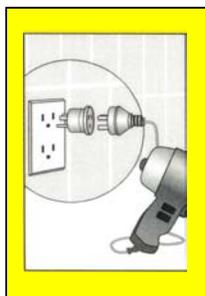
This plug has two flat pins and a round earth and is for use in most parts of North America, Canada, and some parts of South America.
